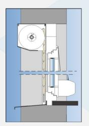
Now the conduit is through the wall and blown free of any dirt or dust you need to fit the cord box and cord roller. Fit the cord roller first. This will fit directly over the hole you have drilled fitted with the roller to the bottom and the brush to the top. The cord box will fit on the wall at about waist height and in line with the roller.
