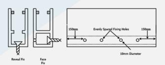
Put the guides back up to the pencil marks and mark on the guide where you require your fixings to be (recommended fixings approx 100mm from top and bottom then fixings equalled out in between, minimum of 3 fixings; average of 300mm between fixings.)
