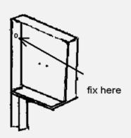
8. Fix the lid on using 4mm rivets using the prdrilled holes. We recommend sealing all around the shutter with a silicone seal.
