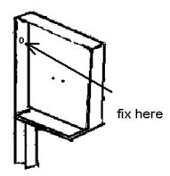
7. Lower the curtain into the guides by feeding the bottom of the curtain over the top of the shaft, then, when the curtain is half way, slide on your t-springs or autolocks. Once the curtain connections are on, carefully lower the curtain all the way down then attach the t springs or autolocks to the shaft as shown in the diagrams below.
