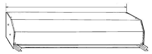
1. First, measure the complete shutter box, and then, using a tape measure, equalise that width across the wall above the window. Mark either end of the intended location of the shutter on the wall with a pencil.
