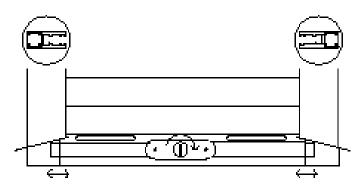
Spring loaded shutters include a transverse lock fitted into the bottom slat. The central key throws out locking bars which locate into the box section of the guide rail at each side.
