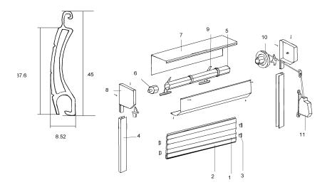
Maximum width: 2000mm Maximum height: 3000mm Maximum square meters: 3m Weight per square meter: 7.3kg
