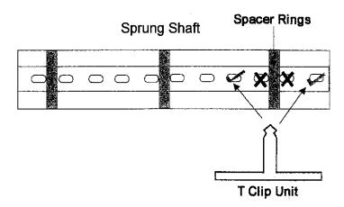
More tension may be required on the spring to assist the raising of the shutter; you can do this by disconnecting the top of the curtain from the shaft and manually rotating the shaft in the direction of the arrow. More turns on the shaft increases the amount of tension. It may take 2-3 attempts to achieve the right balance of tension in the barrel so that it raises the curtain with the right amount of power while allowing you to lower it, too.
